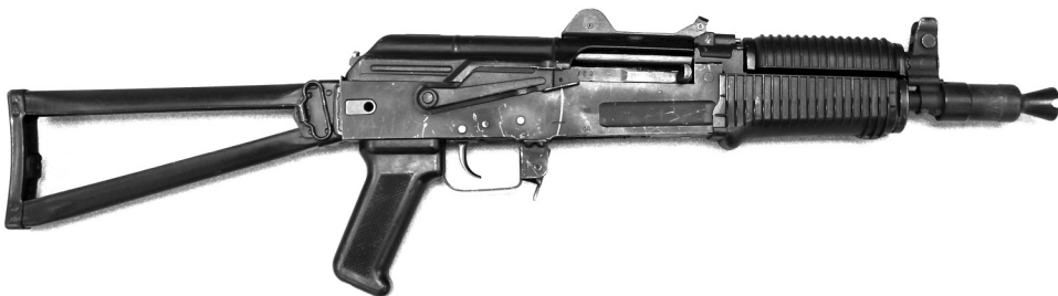
Figure 4.16 A semiautomatic copy of a Russian Krinkov, an AK variant. This exhibit is not a machine gun, it is a short-barreled rifle because of the shoulder stock and barrel that measures approximately 8.5 inches. The weapon was assembled using a parts kit mated to a U.S.-made receiver. (Image from author’s collection.)
